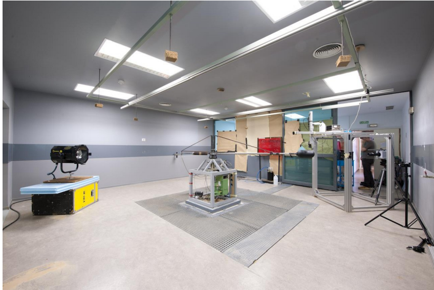
Fig: Experimental rotating arm facility used to verify the analytical model (taken from [1]).
